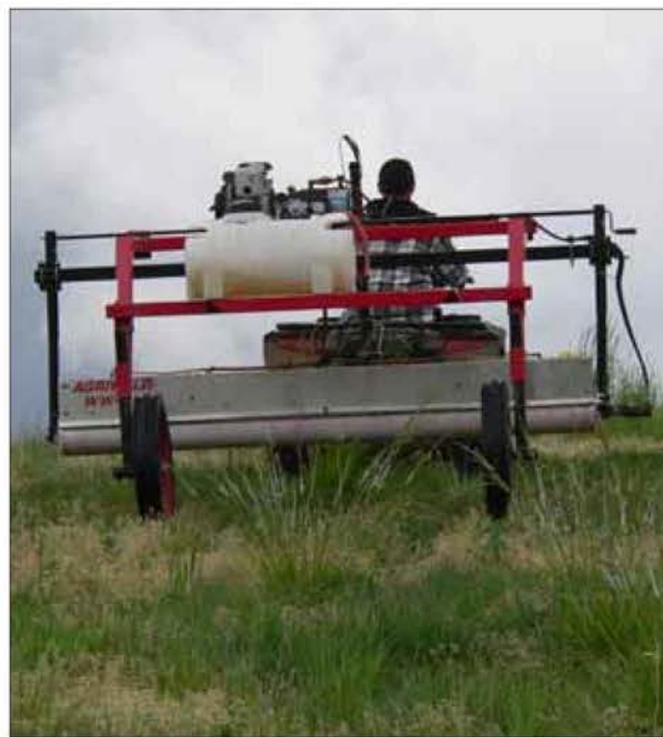
Pesticides should always be applied with care. For herbicides, equipment such as a weed wiper allows more precise application, avoiding nontarget plants and spray drift. (Photograph © Heritage Seedlings/Lynda Boyer.)
